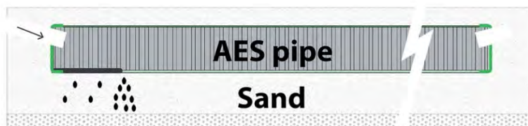
Figure 2. Biofilm build up in AES pipes
